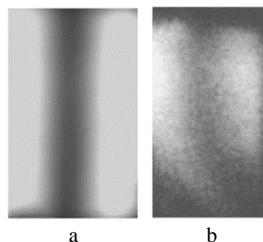
Fig. 2. The spatial intensity distribution at the output of the analyzer for glucose solution (a), and for the drug solution "Inulin-nutrymed" (b)
