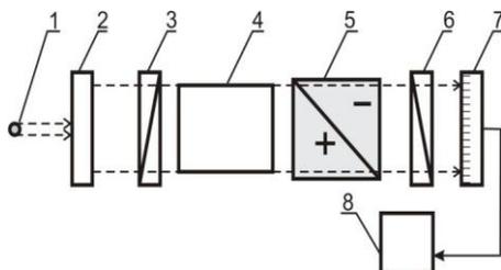
Fig. 1. Block diagram of video polarimeter: 1-light source, 2-extender of beam of light, 3-polarizer, 4-sample cell with investigated optically active material, 5-spatial modulator, 6-analyzer, 7-matrix photodetector, connected to 8-computer interface.
