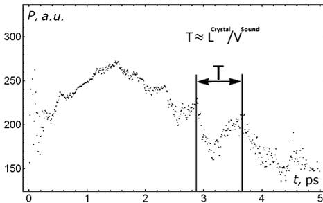
Fig. 1. The time-dependence of crystal dipole moment during its rupture.
