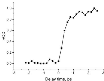
Fig. 1 Time profile of transient absorption for photochromic diarylethene molecules (closed isomer) solved in ethanol solution for the pumping parameters of femtosecond Ti:Sapphire laser:  $\lambda_{\text{pump}} = 266$  nm,  $\tau_{\text{pump}} = 140$  fs.
