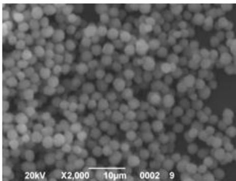
Fig.1. SEM image of synthesized  $\text{CaCO}_3$  microparticles.
