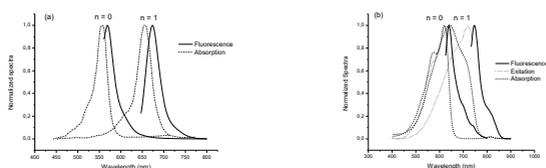
Fig. 2. Normalised absorption, fluorescence and fluorescence excitation spectra of dyes **1** (a) and **2** (b) in acetonitrile.
