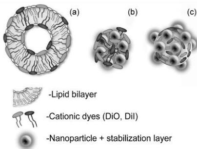
Fig. 1. Schematic representation of PC liposomes/dyes (a) NPs/dyes (b) and NPs/dyes/cholesterol complexes
