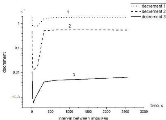
After 60 s photoinduction with light intensity of 6 mW/m<sup>2</sup> RC returns to the dark-adapted state in 500 s after turning off the light. There is a significant slowing down of the relaxation kinetics in the RC recovery process when intervals between light impulses are less than 40 s. After dual photoinduction without interval electron return is
