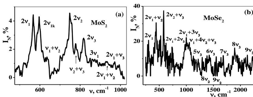
Fig. 1. A series of overtones of main vibrational bands in Raman spectra of natural  $\text{MoS}_2$  (a) and synthetic  $\text{MoSe}_2$  (b), normalized on the intensity of  $\text{A}_{1g}$ .
