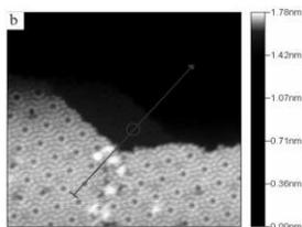
Fig. 1b) STM imaging of the surface of the silicon single crystal with the structure of 7x7 after heating to a temperature of 400 °C.
