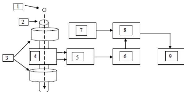
Fig.1. Experimental facility schematics (1 – glass ball; 2 – glass cylindrical cuvette with the regarded system; 3 – windings of electromagnet; 4 – monoblock, containing two pairs light emitting diode (LED) – phototransistor ( $\Phi T$ ). Each pair LED and PT are placed in the apertures of monoblock one against another, and the measuring beam is registered on the other side by PT after passage through the cuvette.
