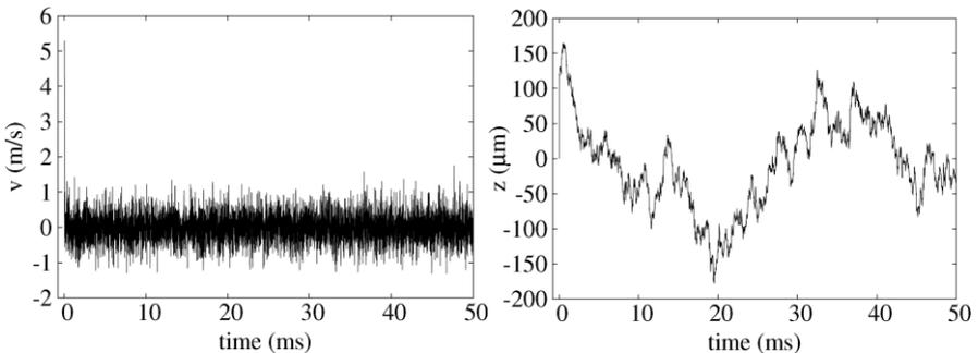
Fig. 1. Dependence of Na atom velocity and coordinate on time. Rabi frequency of each wave is 100 MHz, difference of wave frequency is 200 MHz, red detuning of the average frequency from the atomic transition frequency equals 5 MHz.
