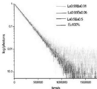
Fig. 1. The luminescence decay curves recorded at 77 K
