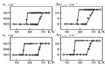
Fig. 2. Change of frequency ( $\nu$ ) and width ( $\Delta\nu_{1/2}$ ) of diphenyl at phase transition liquid-crystal in cycle heating-cooling at cooling rates of 0.4 (a) and 2 grad/min (b).
