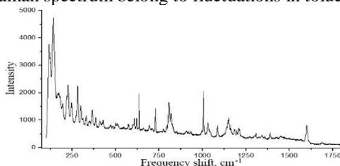
Fig. 3 Raman spectra for a mixture of **α**, **β** and **γ** polymorphs of compound C<sub>18</sub>H<sub>17</sub>F<sub>3</sub>N<sub>2</sub>O<sub>4</sub>S.
