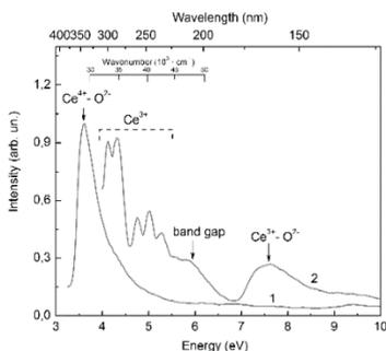
Fig.1. Excitation spectra of oxygen-deficient CeO<sub>2-x</sub> nanocrystals at T=10K, 1- $\lambda_{\text{reg}}$ =630 nm, 2- $\lambda_{\text{reg}}$ =390 nm.
