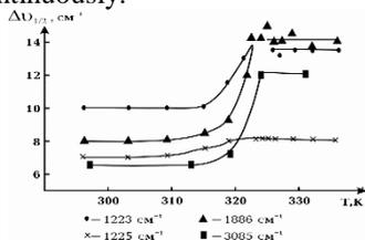
Fig. 1. The dependence of IR bandwidth of diphenyl on temperature in heating cycle in the vicinity of a phase transition liquid-crystal.
