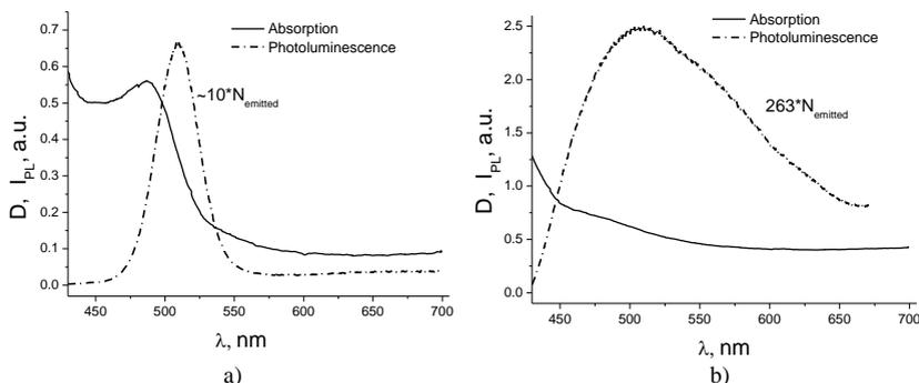
Fig.1 Photoluminescence and absorption spectra of hexane solution of photo-etched CdSe nanoparticles (a), the same solution without photo-etching (b).
