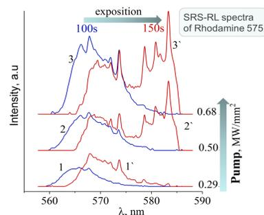
Fig2. Dependence of rhodamine 575 SRS-RL spectrum on vesicles number (proportional to UV exposition under film fabrication) and pumping intensity.
