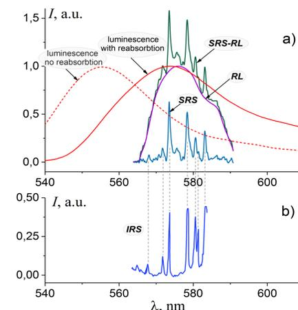
Fig5. a) Disposition RL (violet) and SRS-RL (green) spectra relative to luminescence ones (red) with reabsorption (red solid) and without reabsorption (red dotted) of rhodamine 6G in polymer film; blue line - SRS spectrum evaluated from SRS-RL one. b) Invers Raman scattering (IRS) of rhodamine 6G [5].
