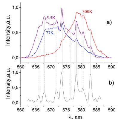
Fig4. a) Dependence of SRS-RL spectrum of rhodamine 6G on temperature. b) Stokes spectrum of Raman scattering obtained by SERRS [4].
