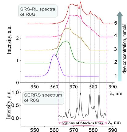
Fig3. Dependence of SRS-RL spectrum of rhodamine 6G on dye concentration under maximal vesicles number (top) and Stokes spectrum of Raman scattering obtained by SERRS [4] (bottom).
