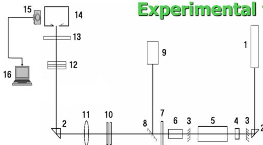
Fig.1. Scheme of laser setup: 1 – He-Ne laser, 2 – rotating prism, 3 – resonator mirrors, 4 – Q modulator, 5 – active element solid-state laser, 6 – frequency doublers, 7 – filter, 8 – half mirror, 9 – calorimeter, 10 – neutral filters, 11 – lens, 12 – dye-doped CLC, 13 – filter, 14 – spectrograph, 15 – video camera, 16 – computer.
