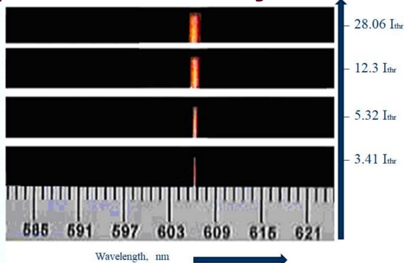
Fig. 4. Spectral characteristics of lasing in the steroidal CLC with orthogonal director orientation on the substrates. The layer thickness  $45 \mu\text{m}$
