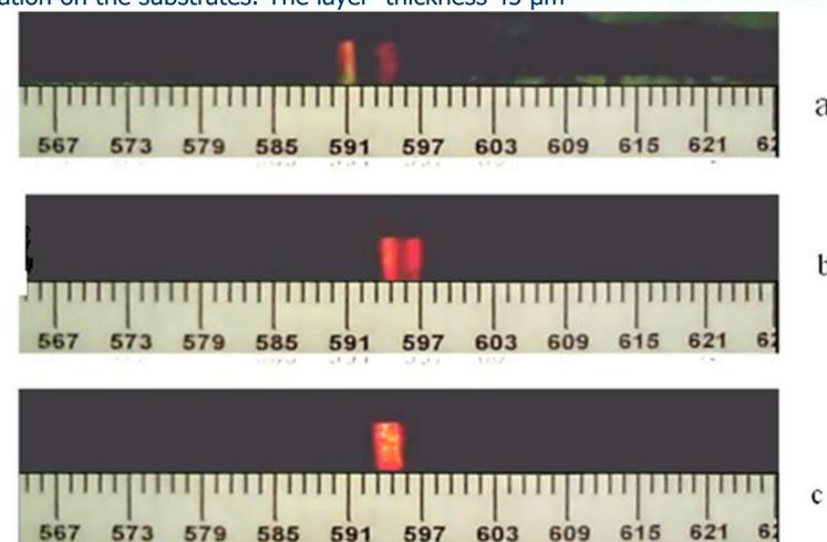
Fig.5. The lasing spectra in steroid CLC activated by phenalene dye F 490 at: parallel orientation with a layer thickness of  $25 \mu\text{m}$  (a); parallel orientation with a layer thickness of  $50 \mu\text{m}$  (b); introduction into the texture of the isotropic glass layer (c).
