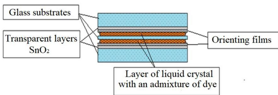
Fig. 2. Scheme of the active element of the CLC laser based on impurity CLC with an isotropic defect in the form of a glass plate.
