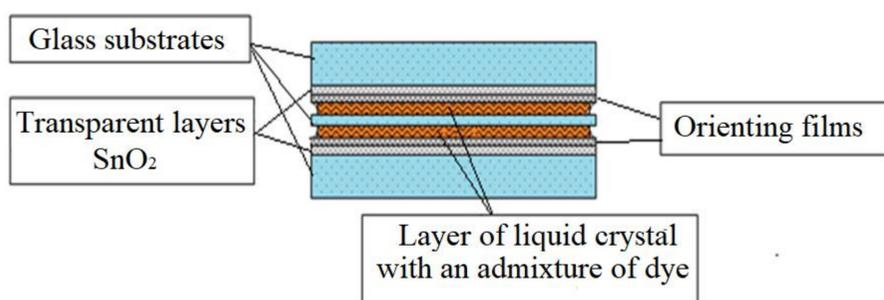
Fig. 2. Scheme of the active element of the CLC laser based on impurity CLC with an isotropic defect in the form of a glass plate.
