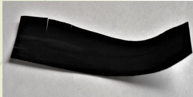
Fig.1. The image of tellurium / tin dioxide nanocomposites printed on the paper substrate
