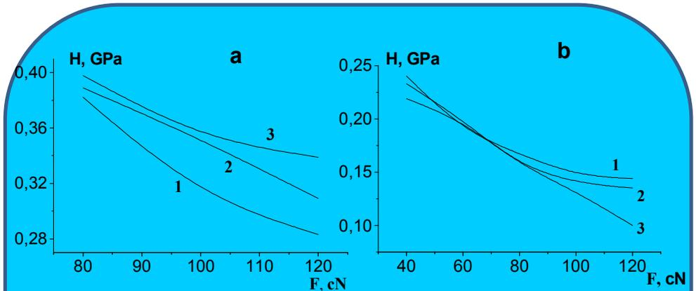
Fig. 1. Dependence of microhardness on the loading on the indenter: a - for samples FP-EG, C (EG) = 3 vol.%, d = 40 (1), 80 (2), 260 (3)  $\mu\text{m}$ ; b - for pure FP (1) and NCM C (EG) = 10 vol.%, d = 120 (2), 500 (3)  $\mu\text{m}$ .
