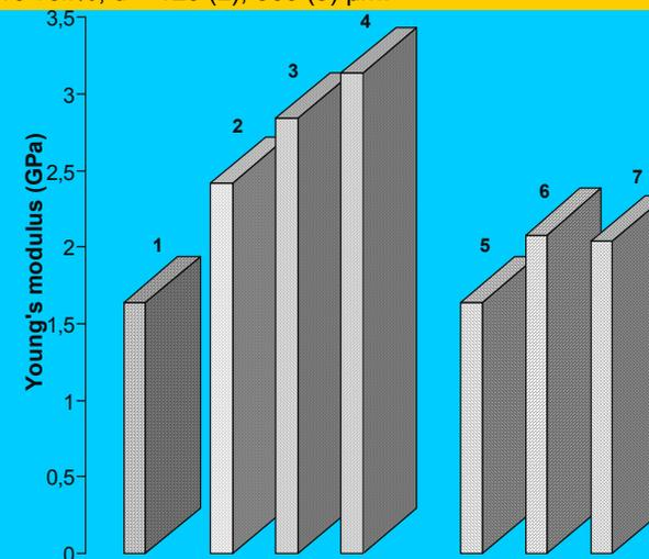
Fig. 2. Young's modulus for samples of FP (1) and NCM FP-EG. The concentration of EG is 3 vol.% (2, 3, 4) and 10 vol.% (5, 6, 7) and the dispersion of its particles 40 (2), 80 (3), 120 (5), 180 (6), 260 (4) and 500 (7)  $\mu\text{m}$ .
