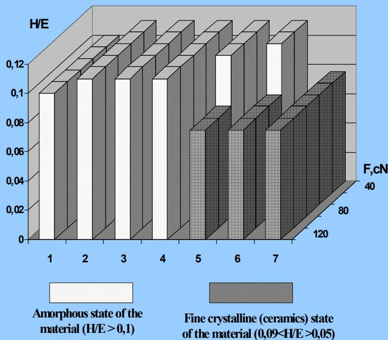
Fig. 3. Dependence of the  $H/E$  ratio at different degrees of load for samples of FP (1) and NCM FP-EG with a concentration of EG 3 vol.% (2, 3, 4) and 10 vol.% (5, 6, 7) and dispersion of its particles: 40 (2), 80 (3), 120 (5), 180 (6), 260 (4), 500 (7)  $\mu\text{m}$ .
