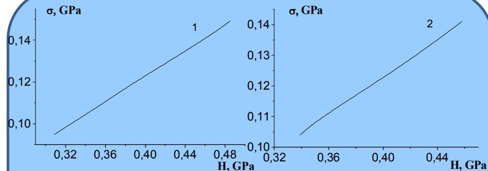
Fig. 4. Dependence of the magnitude of the stress, which corresponds to the onset of plastic deformation of the material under tension on the microhardness obtained using the Micron-gamma device for the FP-EG samples ( $C(EG) = 3 \text{ vol.}\%$ ,  $d = 40 \mu\text{m}$  (1),  $260 \mu\text{m}$  (2)).
