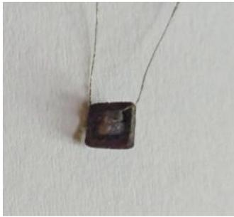
Figure 1. The formed sample of  $\text{GaSe}\langle\langle\text{NaNO}_2\rangle\rangle+\langle\text{FeCl}_3\rangle\rangle$  clathrate.
