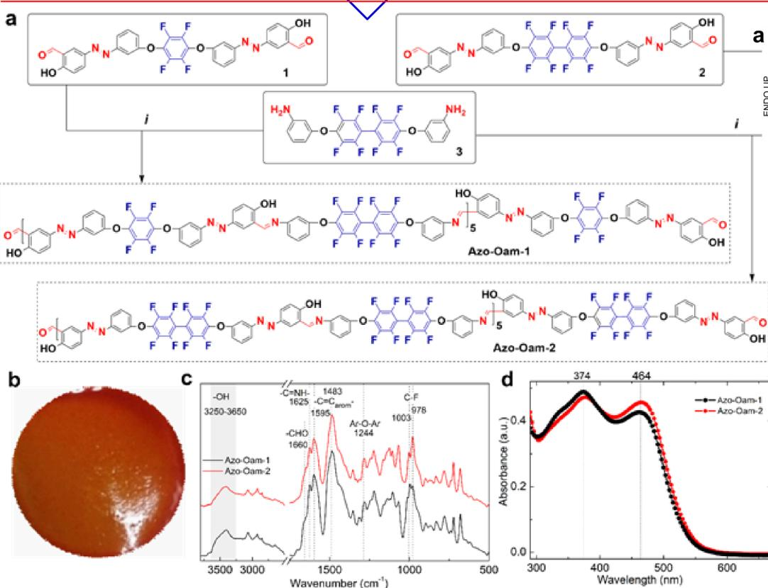
Figure 1. a) Synthesis of Azo-Oam-1 and Azo-Oam-2 oligomers: (i) DMAC, 110 °C, 24 h. Yield about 86% for both oligomers after reprecipitation. b) Digital image of self-standing Azo-Oam-2 oligomer (thickness 100 μm). c) FTIR spectra of synthesized Azo-Oam oligomers; d) UV-vis absorbance spectra of oligomers Azo-Oam-1 and Azo-Oam-2 in DMAC (0.006 mg/mL).
