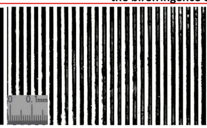
Figure 8. The photo of a diffraction grating Azo-Oam-1 film in polarization microscope,
