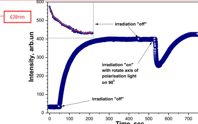
Figure 5. The dependence of the intensity of the "test" beam when changing the birefringence on the time of irradiation of polymers Azo-Oam-1
