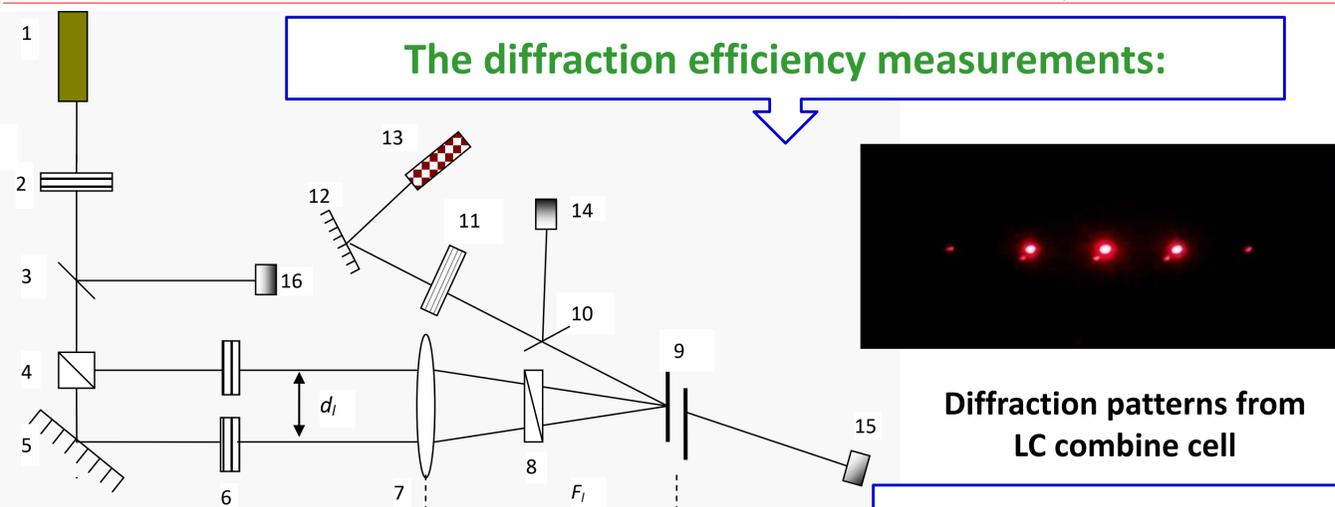
Experimental set-up: 1 – DPS Laser ( $\lambda = 532 \text{ nm}$ ); 2 –  $\lambda/2$ -waveplates; 3, 10 – beam-splitter plates; 4 – beam-splitter cube; 5, 12 – mirrors; 6, 8, 11 – polarizer; 7 – lens; 9 – sample; 13 – He-Ne laser ( $\lambda = 632.8 \text{ nm}$ ); 14, 15, 16 – photodiodes.
