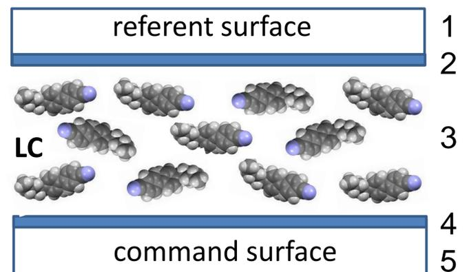
Scheme of LC cell: 1;5-glass substrate, 2 – referent layer; 3 – liquid crystal; 4 – command layer (ITO, nano-gold island, chalcogenide)
