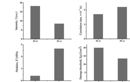
Relative integral intensity of TEMPO spectra (I) and pmp correlation time ( $\tau$ ) agree with storage modulus ( $E'$ ) and threshold of single-pulse laser damage ( $E_d$ ) in the polyurethane matrices based on OPG-1000 and different diisocyanates
