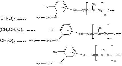
PU-4 aromatic diisocyanate - toluene diisocyanate (TDI), bifunctional oligoether diol – OPG-1000 and TMP
