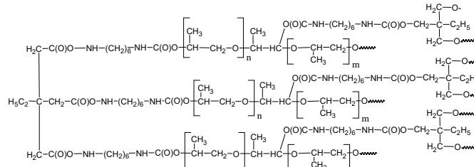
PU-1 aliphatic diisocyanate – hexamethylene diisocyanate (HMDI), trifunctional oligoether triol – oligo-oxypropylene glycol with MM 500 (OPG-500), trimethylolpropane (TMP)
