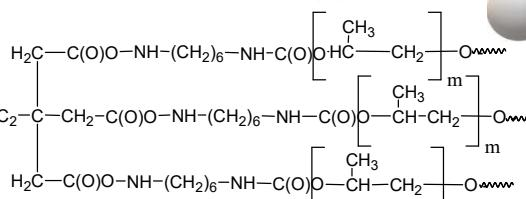
PU-2 aliphatic diisocyanate HMDI, bifunctional oligoether diol – oligo-oxypropylene glycol with MM 1000 (OPG-1000), TMP
