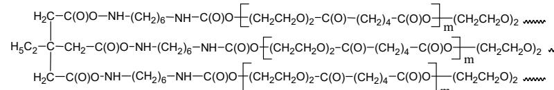
PU-3 HMDI, bifunctional oligoester diol – oligo-diethylene glycol adipate with MM 800 (ODA) and TMP
