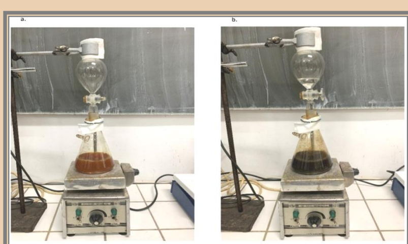
Fig. 1 Reaction vessel, on heating plate before hot NaOH adding (left) and after that when black MNP in suspension (right).
