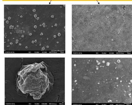
In the sample synthesized by method 1, the vanadate nanoparticles are grouped together and arranged in separate islands. The samples obtained by method 2 are characterized by homogeneous structure. They do not have filamentous fragments and inclusions of another type. These samples are characterized by a granular structure sometimes with a low pore content. The grain sizes are about 20 nm.
