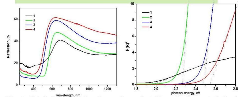
Using the Kubelko-Munch transformations, we have estimated from reflection spectra the band gap of synthesized vanadate-borate glass composites by determining of tangent versus photon energy to the  $F^2$  curve, where  $F = (1-R)^2/2R$ ,  $R$  is the reflection spectrum.
