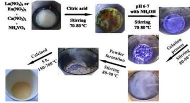
The initial luminescent  $\text{La}_{1-x}\text{Eu}_x\text{Ca}_y\text{VO}_4$  nanoparticles were synthesized by sol-gel method from calculated stoichiometric amounts of  $\text{La}(\text{NO}_3)_3$ ,  $\text{RE}(\text{NO}_3)_3$ ,  $\text{NH}_4\text{VO}_3$ ,  $\text{Ca}(\text{NO}_3)_2$  precursors by sol-gel method.
