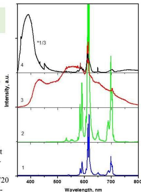
Narrow line  $\text{Eu}^{3+}$  emission is strongly suppressed for the  $90\text{B}_2\text{O}_3\text{-}3\text{V}_2\text{O}_5\text{-}3\text{La}_{0.8}\text{Eu}_{0.1}\text{Ca}_{0.1}\text{VO}_4\text{-}4\text{ZnO}$  samples.
