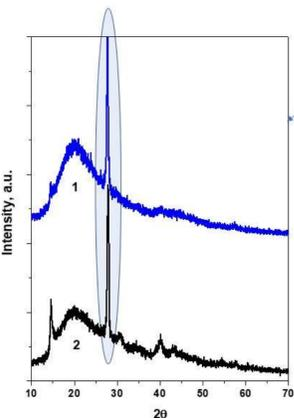
The XRD patterns of the  $94\text{B}_2\text{O}_3\text{-}3\text{V}_2\text{O}_5\text{-}3\text{La}_{0.8}\text{Eu}_{0.1}\text{Ca}_{0.1}\text{VO}_4$  composites made by methods 1 (1) and 2 (2)
